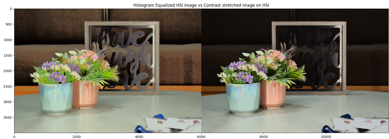
Figure 38: Histogram Equalized image on HSI vs Image stretched on HSI channel
