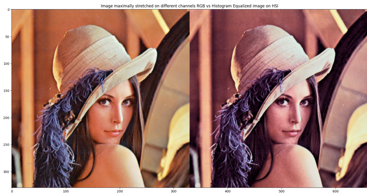
Figure 39: Image maximally stretched on different channels RGB vs Histogram Equalized image on HSI
